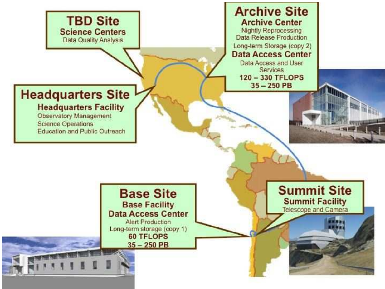
FIG. 17.— The LSST data flow from the mountain summit/base facility in Chile to the data access center and archive centers in the U.S.
