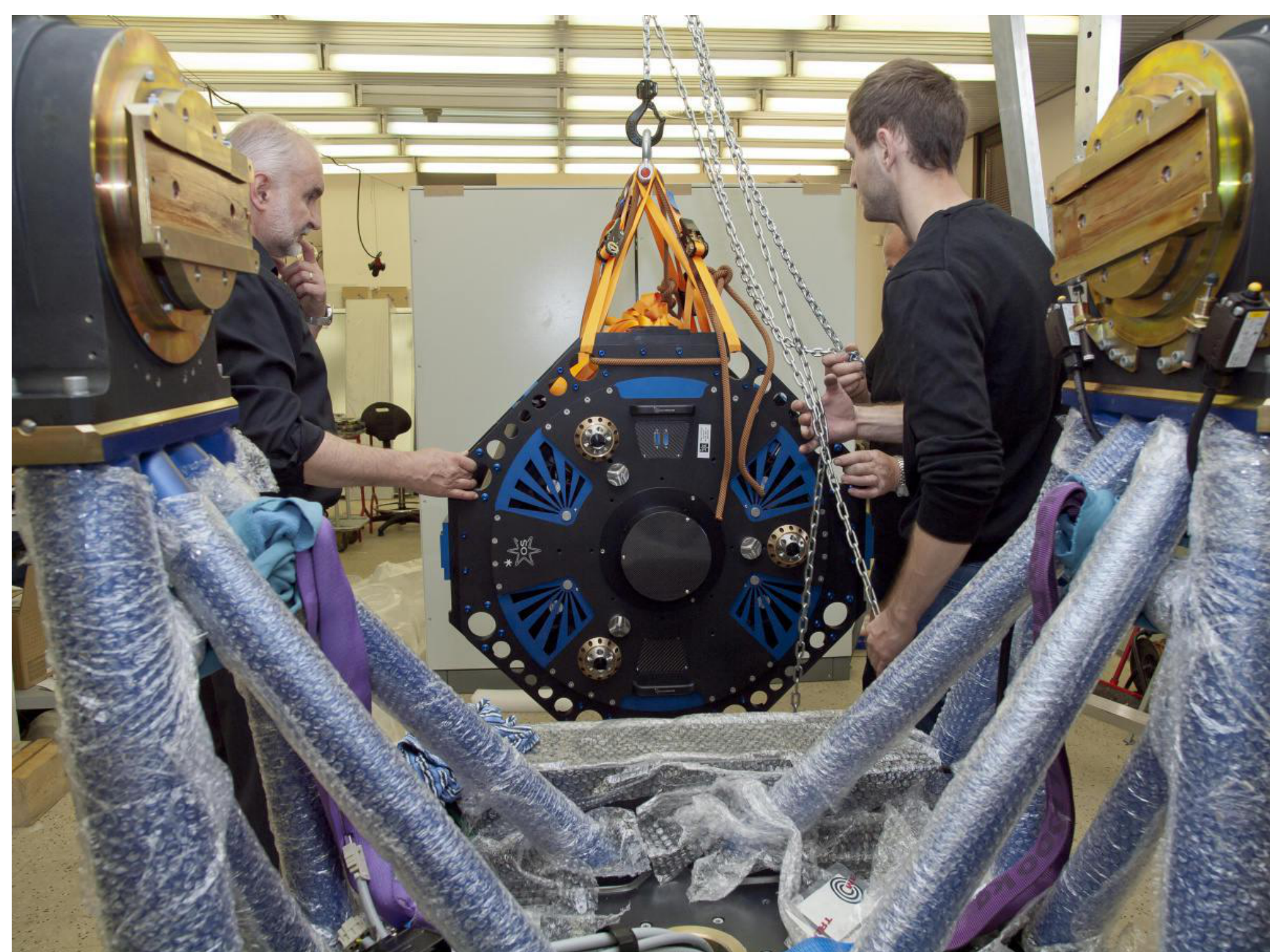
Figure 3: An ongoing completion of the alt-azimuth mount (to be equipped with Officina Stellare RiLA 600 f/5 reflector, MI CCD camera with an E2V chip 42-20-BI, >90% QE, FOV 0.52 deg). Most of the electrical equipment (including UPS power supply) is located in a separate container. The place at the Ondřejov observatory is ready.
