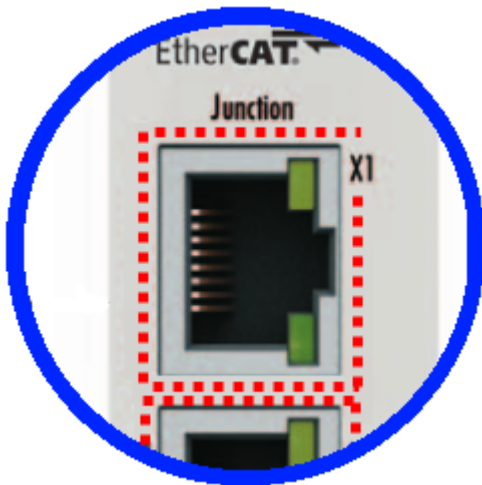
Fig. 10: Identification of FHC port at EK1122-0080 and EK1101-0080
