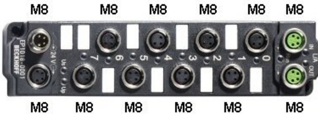
Fig. 34: EtherCAT Box with M8 connectors
