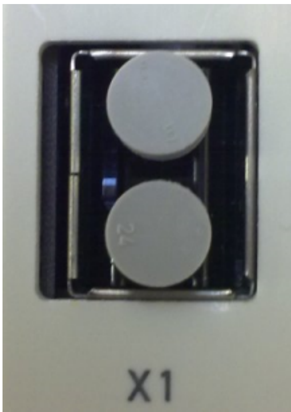
Figure: Blind plugs in unused sockets
