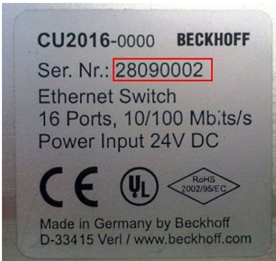
Fig. 3: CU2016 switch with serial/ batch number
