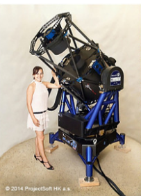
Figure 3: An optimisation of the alt-azimuth mount during the development phase. The final mount equipped with Officina Stellare RILA 600 f/5 reflector and a sensitive CCD camera (EZV chip 42-20-BI, >90% QE, FOV 0.52 deg). The complete autonomous observatory is now located in Ondřejov, Czech Republic. The first-light image (M31)!
